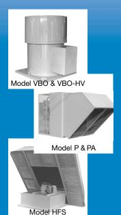
**MODEL VBO-HV** – Available with U.L. Listing for "Power Ventilators For Smoke Control Systems". Heat and smoke exhauster is designed to meet the high temperature requirements of the Uniform Fire Code and IRI recommendations. Independently tested to operate without failure at 500°F for a minimum of 4 hours, and 1,000°F for a minimum of 15 minutes.
