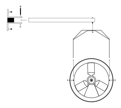
6. Check fan rotation upon startup. Standing in front of fan, the blade should be turning clockwise. If rotation needs to be reversed this usually can be accomplished by reversing the connection wires.
